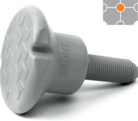
The connecting pin is what holds the cubes together, once inserted into the sliding nut. When fixed in its position, the connecting pin, which also features anti-slip surface, becomes a part of the dock and contributes to the overall stability of the system.
